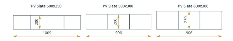
Dimensions show the visible area of a single PV Slate unit on the roof.
